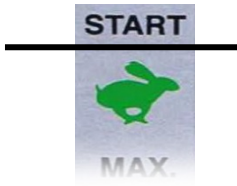
Fig. 11 - Control cold start
