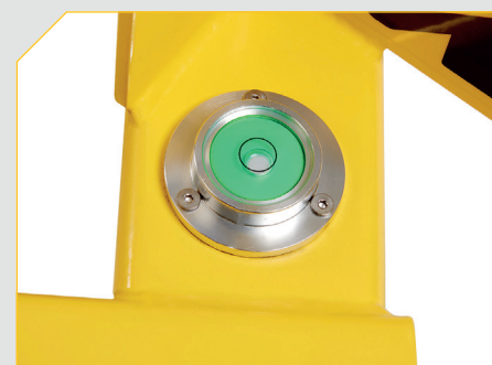
Spirit level to aid the operator to level the chassis.
