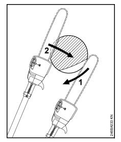
To avoid tearing the bark on thick branches, always start by performing a relieving cut (1) on the underside of the branch.
