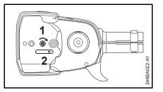
Turn the screw (1) clockwise until the tensioner slide (2) butts against the right end of the housing slot.
