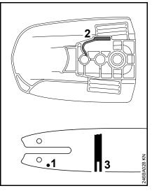
The drive link tangs will otherwise scrape along the bottom of the groove – the cutters and tie straps will not ride on the bar rails.
