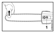
Re-tensioning during cutting work:
