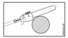
To avoid pinching the bar in the cut, position the cutting attachment with the housing against the branch and then perform the cross-cut from the top downwards.
