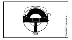
The marks on the cap and oil tank are then in alignment.
