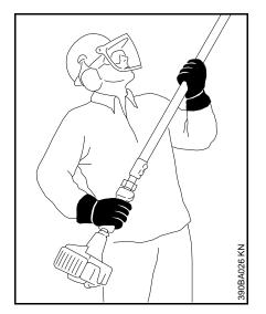
Always hold the unit **firmly with both hands** – right hand on the control handle, left hand on the drive tube – even if you are left-handed. Wrap your fingers around the control handle and drive tube.
