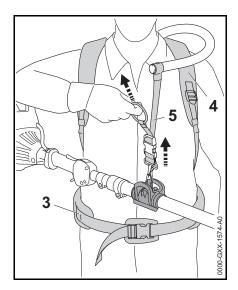
Adjust the hip belt (3), both shoulder straps (4) and the carrying strap (5).
