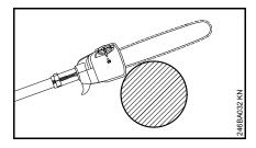
Position the cutting attachment with the hook against the branch and then perform the cross-cut. This reduces the risk of the pruner being jerked forward as you start the cross-cut.
