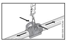
Squeeze the clip together to move it up or down the shaft.
