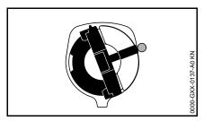
Marks on tank cap and oil tank must line up.
