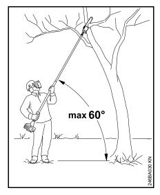
Hold the pole pruner at an angle. Do not stand directly underneath the limb being cut. Do not exceed an angle of 60° from the horizontal. Watch for falling wood.
