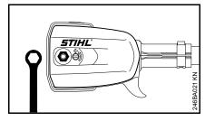
Unscrew the nut and remove the chain sprocket cover.
