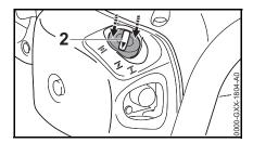
Depress the outer ring (arrows) of the choke knob (2) and then turn it to //.
