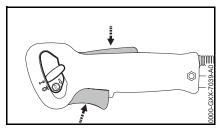
Press down the throttle trigger lockout and open the throttle – the choke knob moves to the run position —. After a cold start, warm up the engine by opening the throttle several times.
