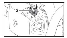
Depress the outer ring (arrows) of the choke knob (2) and then turn it to <u>T</u>.
