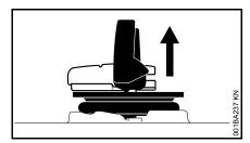
Remove the tank cap.
