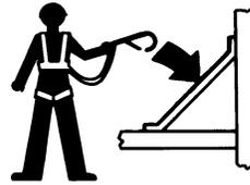
Occupants should wear a safety belt or harness and comply with applicable governmental regulations. Attach the lanyard to the anchor provided in the platform.
