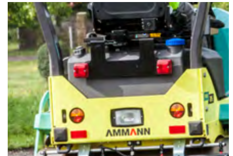
ROAD LIGHTING & REVERSE ALARM
