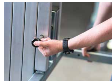
Assembly and fixing of the Load fork using ball lock pins
