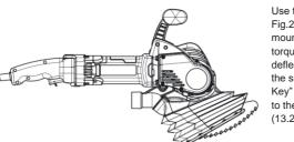
Use the "lan key" (see Fig.2), to tighten the blade mounting screws until the torque indicator coil deflects sufficiently so that the sides meet. The "lan Key" will tighten the bolts to the required 18Nm (13.2 ft lb).
