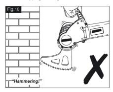
When using the Mortar Plunge blades, the cut should
