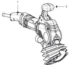
Before changing blades, the guard around the blade mounts must be levered gently out of its groove at the front of the tool and swung away to give access to the cap screws. (See Fig.1)
