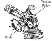
To access these items, remove the 4 screws holding the plastic cover on the right side of the tool (see Fig.14). Inspect the
