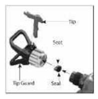
WARNING: Never attempt to spray with the tip in any position in-between either fully forward or fully reversed. It could cause a high pressure hazard.
