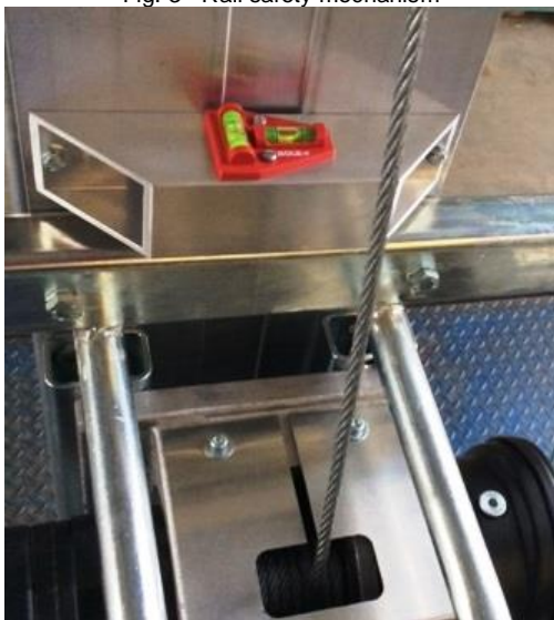
Fig. 5 - Spirit level above winch
