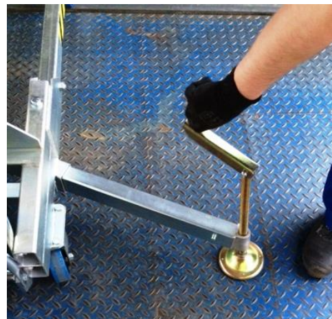
Fig. 6 - Lateral outriggers with spindle
