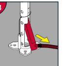
Continue to support outer tube and remove ram via ram access chamber.
