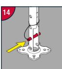
Reinsert bottom pin in its storage position.
