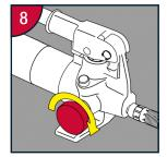
When making ready for storage, ensure flow valve is in the closed position.
