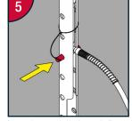
Insert bottom pin through first available hole directly beneath ram.
