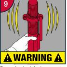
Pump the handle just enough to free up the collar. Do not over-pump.
