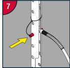
Insert bottom pin through first available hole directly beneath the ram.
