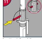
Insert top pin through the available hole in the threaded section above the collar.
