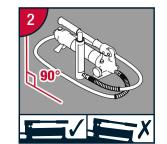
Place Hydraulic Assembly on ground in horizontal position.
