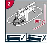
Ensure the Hydraulic Assembly is placed in a horizontal position or it will not function properly.
