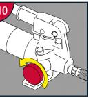
Open flow valve to allow ram stick to retract and inner tube to lower.
