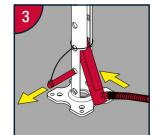
Remove bottom pin and insert ram into ram access chamber.
