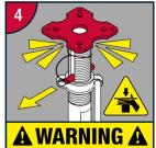
Remove top pin. Inner tube fully retracts. Be aware of trap/crush injuries.
