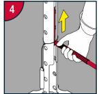
Lift hose to raise ram until ram is as near as possible to inner tube.
