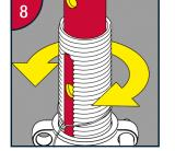
Prior to engaging the pump align holes of inner tube with slot in threaded collar section.
