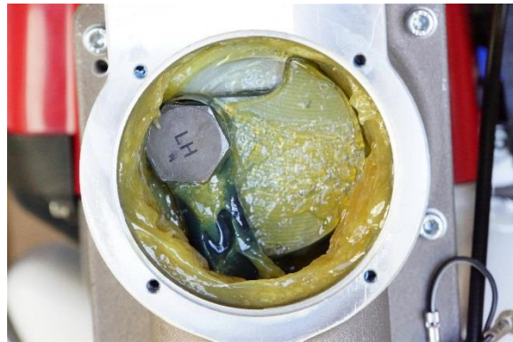
Figure 2 Crank area with sufficient grease. Colour is yellow prior to use as above, and will tend to brown with age and use.
